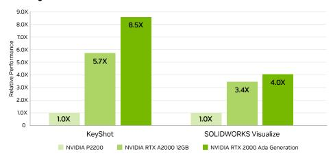
Tests run on an Intel Core i9-12900K Processor @ 3.2GHz (5.2GHz Turbo), 64GB RAM, Windows 11 Enterprise x64, NVIDIA Driver 550.76. KeyShot geomean (time - seconds), SOLIDWORKS Visualize geomean (time) 1080p tests. Performance based on prerelease build, subject to change.
